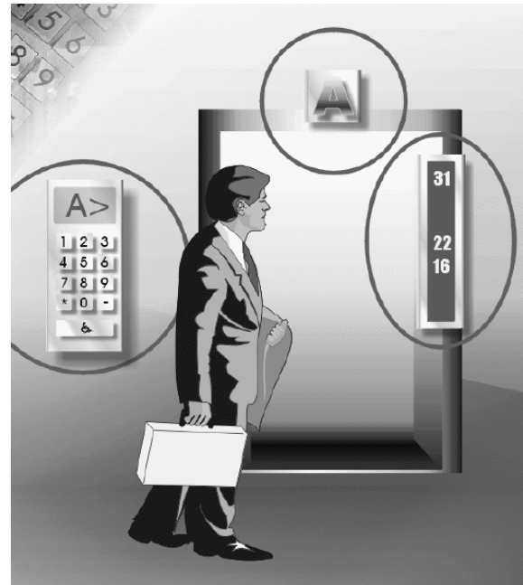
Figure 1: A Miconic-10™ keypad allows passengers to enter their destination before they enter the elevator. A display informs the passenger about the elevator that will offer the most suitable transport.
