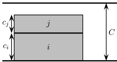
Figure 1: Two tasks i and j of the same family ( f_i = f_j ) can be processed simultaneously.
