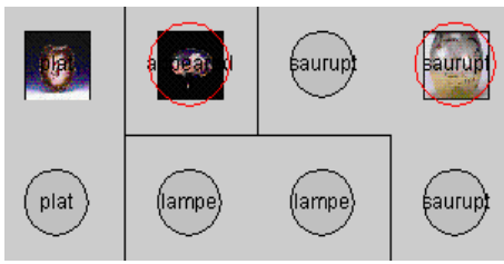
Figure 1: Partial view of a topographic Kohonen map: icons show the most representative member of the classes, labels represent class names, circles represent intermediate classes, lines represent logical area borders
