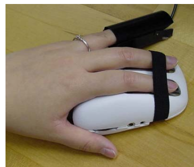
Figure 1: GSR and BVP sensors
