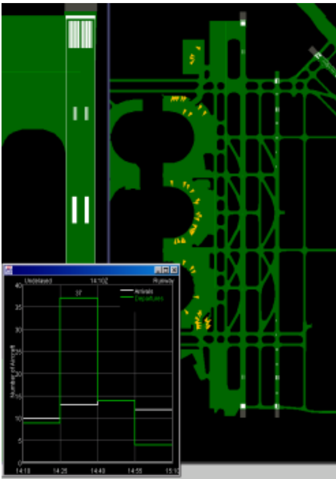
Figure 1: Surface Management System displays: Map of airport showing aircraft locations. Coded data blocks (not shown) display aircraft identification, type and other data. Load graph shows machine-predicted delays at future times; both arrival and departure delays are calculated.
