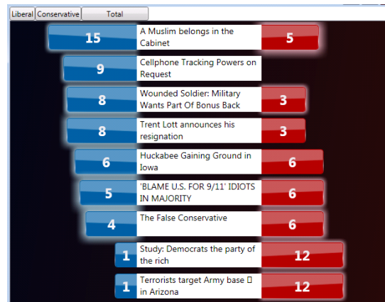
Figure 8: The BLEWS User Interface. “Wings” on each side of the title show the number of in-links to each article; the glow around each article suggests its emotional sentiment. In this view, the display is sorted by number of liberal in-links.
