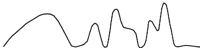
Figure 7. A variety of shapes occur in trace data. Trace data takes on a number of characteristic shapes. Some are sharp curves, some contain a shoulder, and others appear as long smooth curves.
