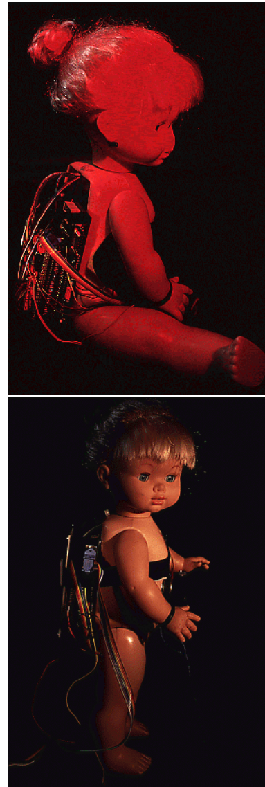
Figure 3: The second prototype of Robota is a standalone robot. It can be connected to a PC for speech and vision-based interaction. The reproduction of the photos are a courtesy of Eurelios.
