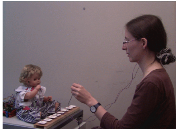
Figure 2: The teacher guides the robot's motions using a pair of glasses holding a pair of IR emitter. The glasses radiation which can be picked up by the robot's "ear-rings" IR receptors.
