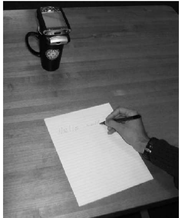
Figure 1: The user writes with an ordinary pen on an ordinary pad of paper. A camera connected to a portable computer (in this case, an iPaq) captures just the strokes along with temporal information, just as if the user were writing on a digitizing table.
