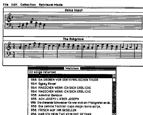
Figure 6. Display from the tune retrieval system
