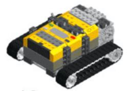
Figure 1. RCX unit. IR port is "in front," at lower left. Sensor ports are gray squares behind the IR port. Output ports are dark squares located beyond the LCD display.
