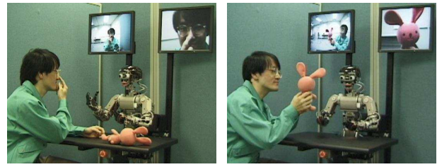
Figure 3: Infanoid , the child-like humanoid robot, engaging in eye-contact (left) and joint attention (right) with a human interactant. (The video monitors behind show Infanoid 's peripheral and foveal views.)
