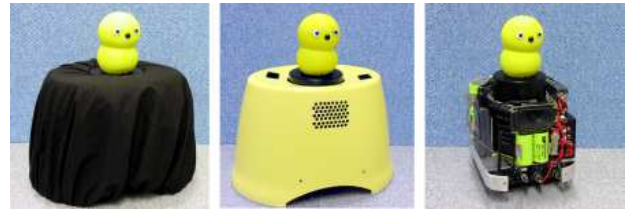
Figure 9: A self-contained version of Keepon , equipped with a battery and wireless connections.
