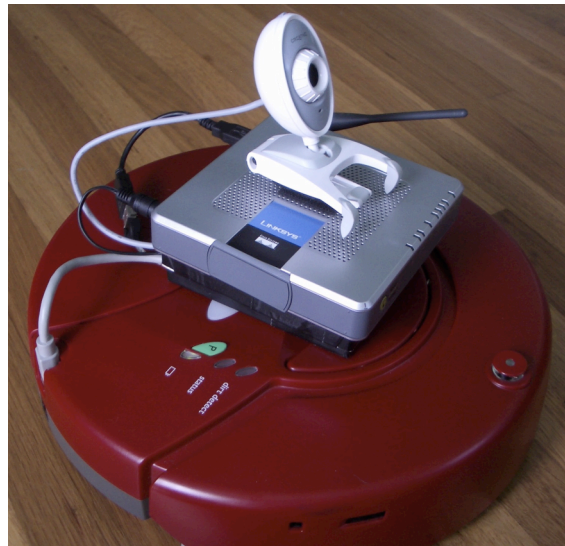
Figure 2 Autonomous Linux Roomba utilizing a WRTSL54GS, USB webcam, flash drive, and serial port.
