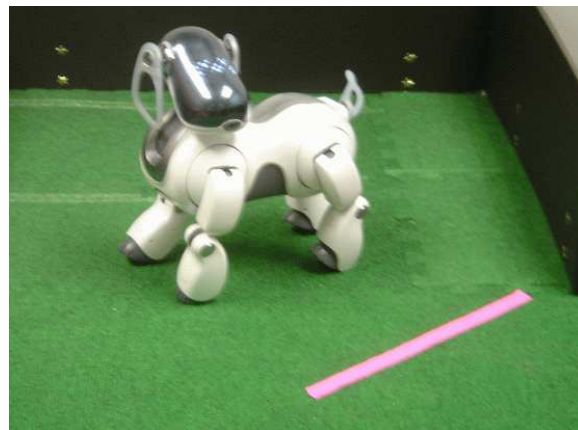
Figure 7: Joint limits constrain motion. In this position, the head can not turn far enough to the left to see both endpoints of the line.
