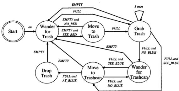
Figure 3: An FSM representing behavior of a trash pickup robot (reproduced from Murphy 2000, p. 181)
