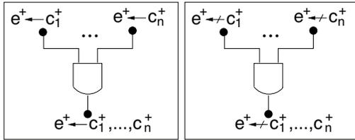
Figure 1: Direct (left) and dual (right) NIN-AND gates
