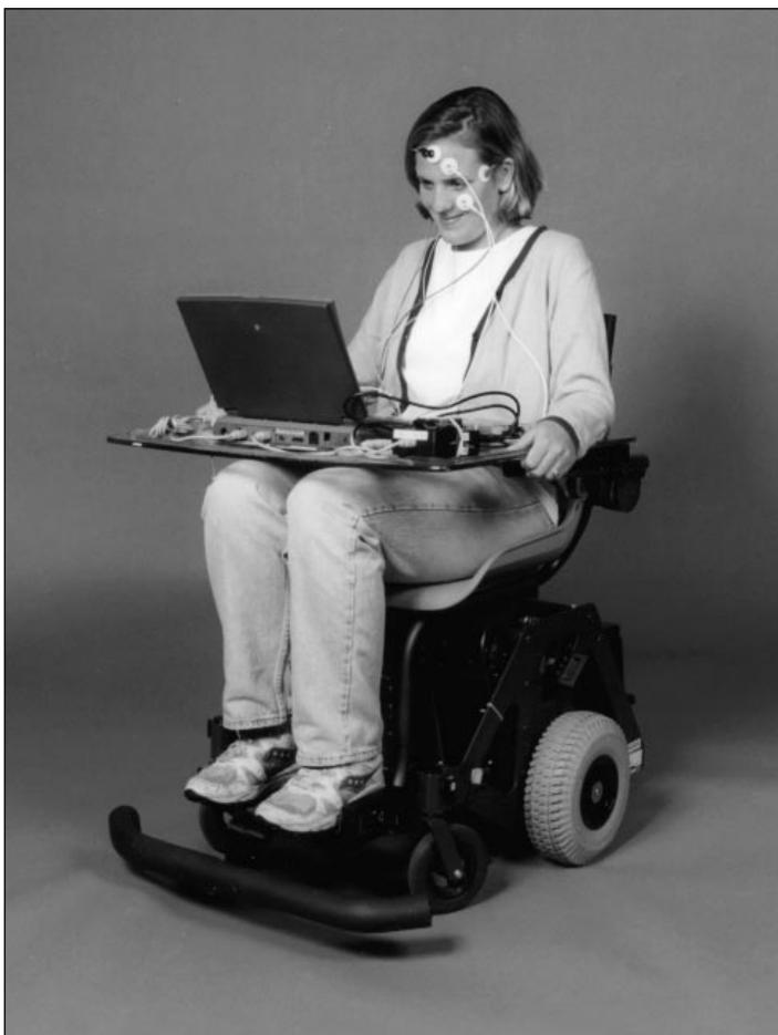
Figure 8. WHEELSLEY, a Robotic Wheelchair from the MIT AI Lab, Receiving Commands from the User through EAGLEEYES, an Eye-Tracking System from Boston College.
