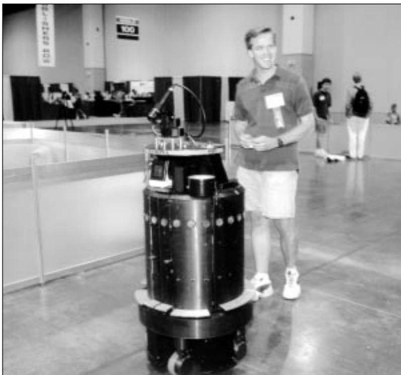
*Figure 6. Brown University's RAMONA Uses Optical Flow to Wander in Complex, Cluttered Environments at Speeds as High as 50 Centimeters/Second.*
