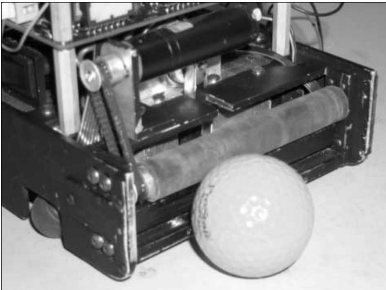
*Figure 5. Angled View, Dribbling Mechanism.*
