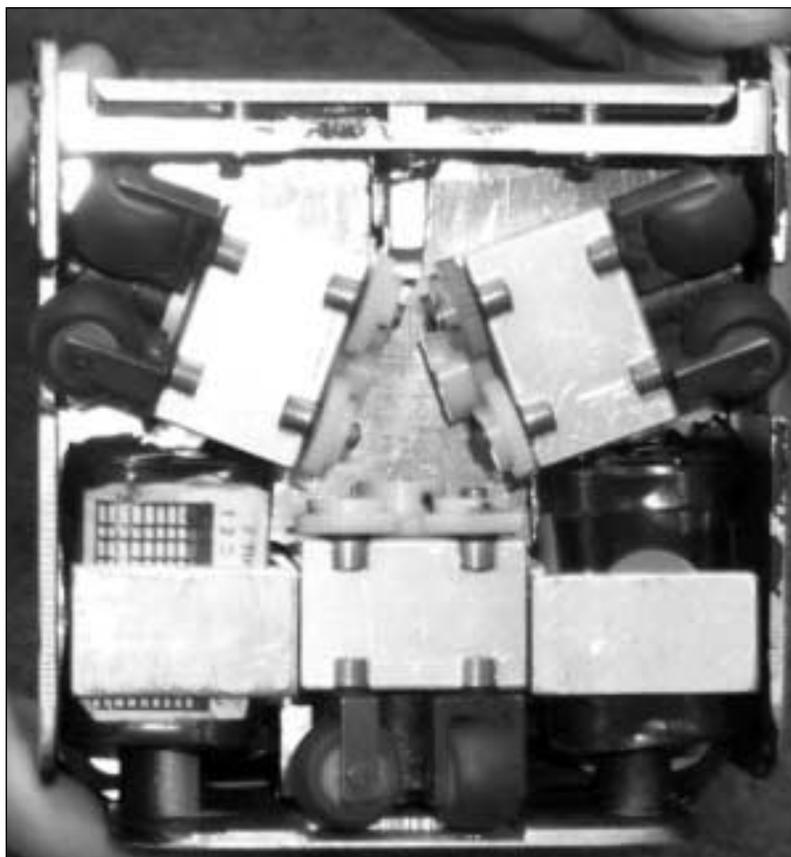
Figure 4. Bottom View, Omnidirectional Drive.
