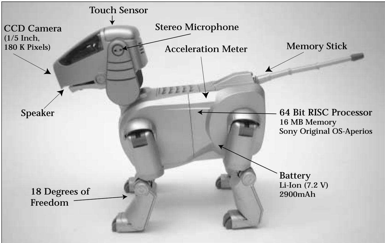
Figure 1. The Legged Robot Platform.
