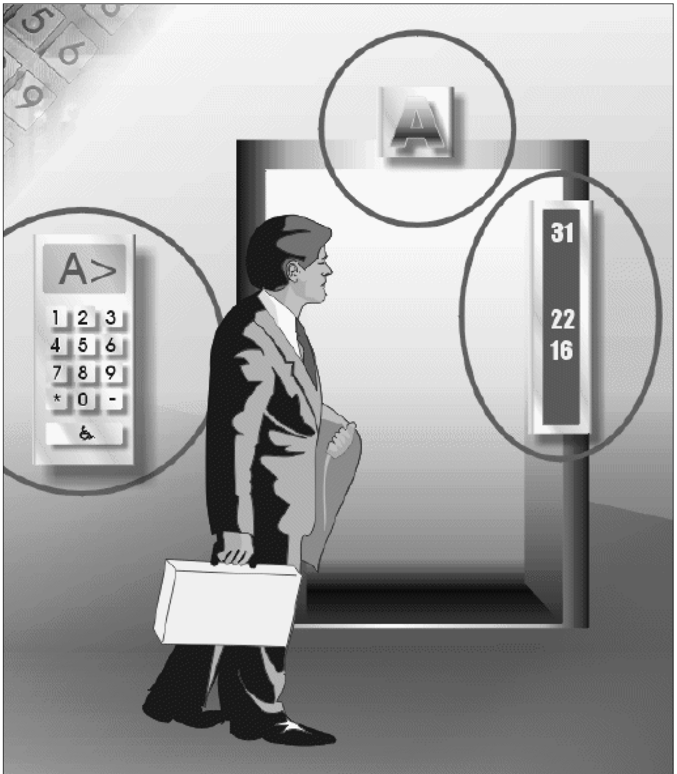
Figure 1. A Telephone-Like 10-Digit Keypad Allows Passengers to Enter Their Destination before They Enter the Elevator. A display informs passengers of the elevator to which they have been allocated.
