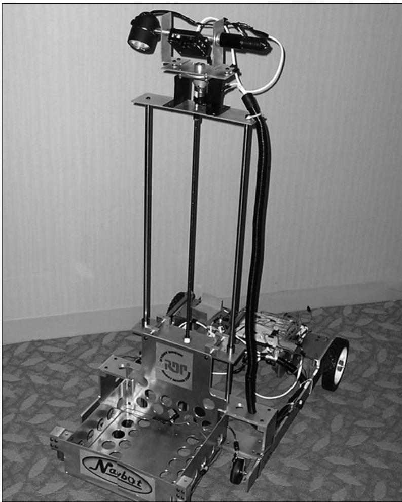
Figure 4. The Custom-Built Scavenger Hunt Robot from the Stony Brook Robot Design Team.
