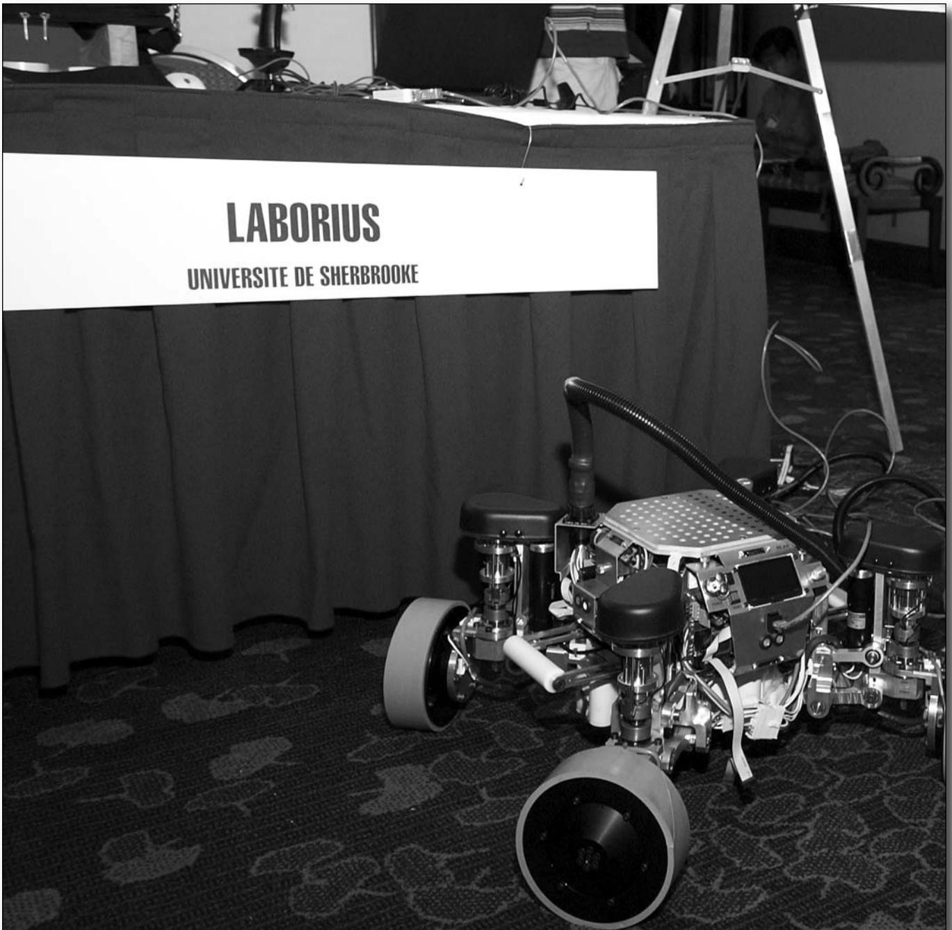
*Figure 16. The Azimut-2 Omnidirectional Modular Platform from the Université de Sherbrooke.*
