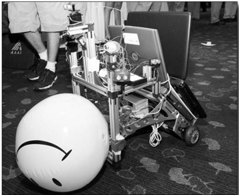
*Figure 2. The Winning Scavenger Hunt Entry from Harvey Mudd College Based on an Evolution Robotics ER-1 Robot Platform.*
