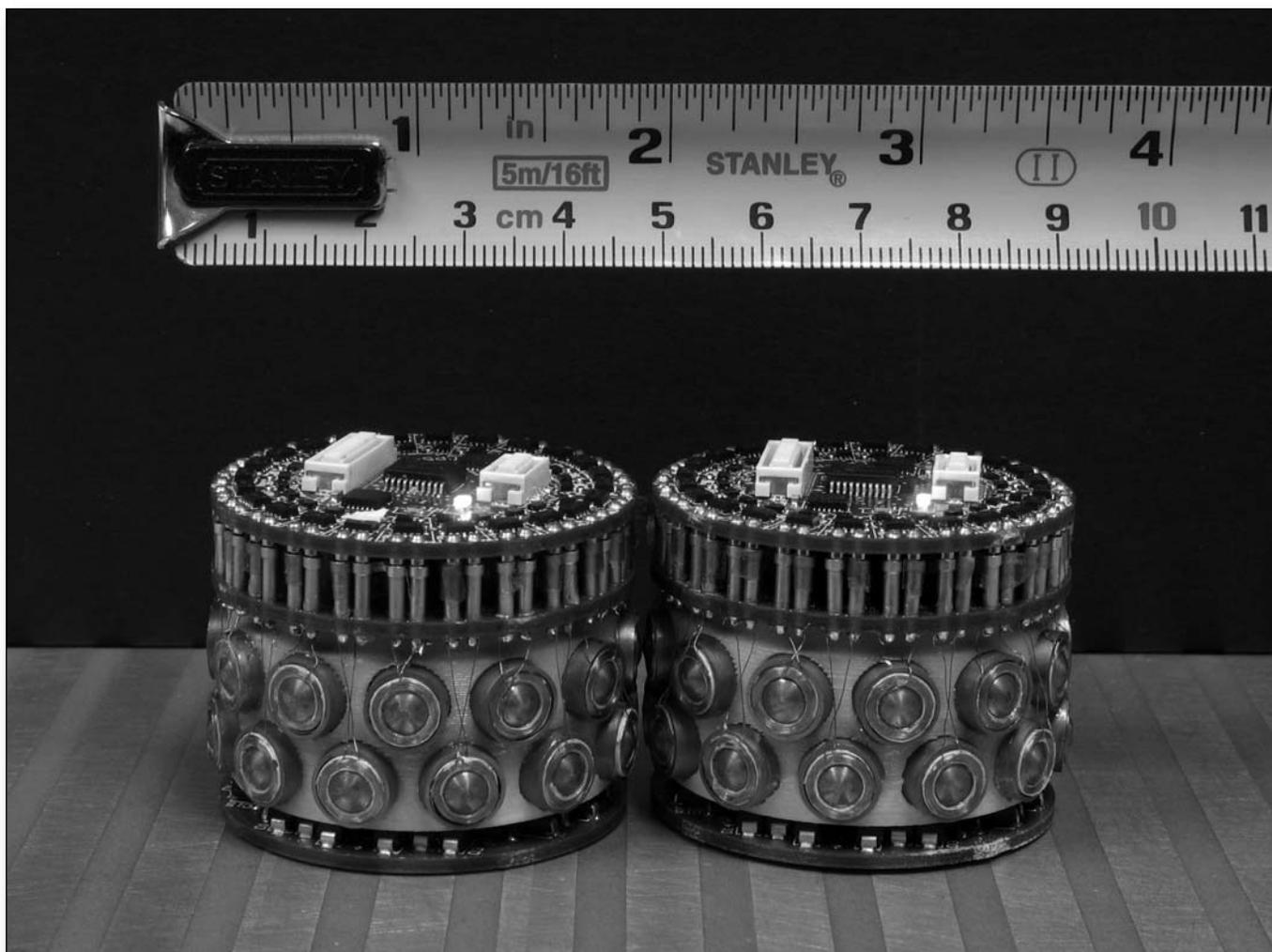
Figure 12. Two Nodes from the Claytronics Project.
