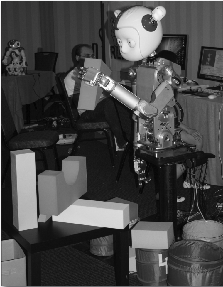
Figure 3. Simon, the Georgia Tech Robot, Sorting Colored Blocks for the Learning by Demonstration Challenge.
