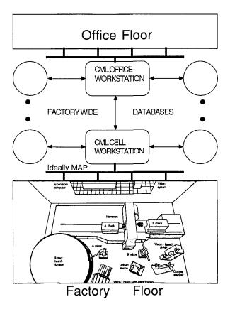
Figure 2. CML's Role in the Manufacturing Environment.
