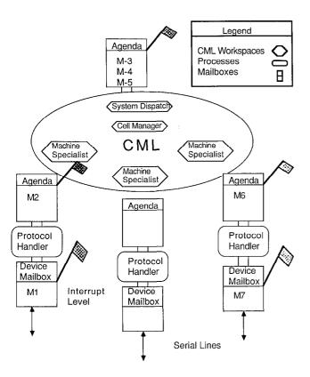
Figure 14. Data Flow in a CML System.
