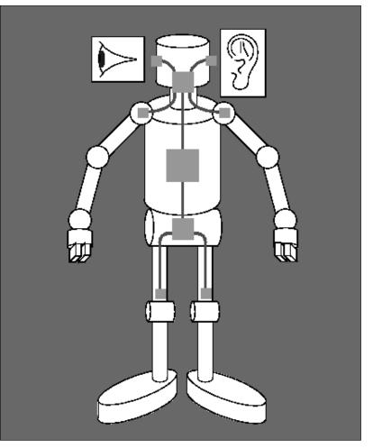
Figure 5. This Robot Design Continues the Progression Started in Figure 4. This architecture allows for sensor-effector control loops that operate with minimal and only intermittent supervision from a centralized computing resource.
