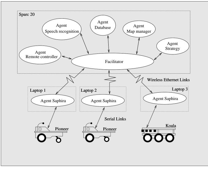
Figure 5. Organization of Physical and Software Agents for the Robot Contest.
