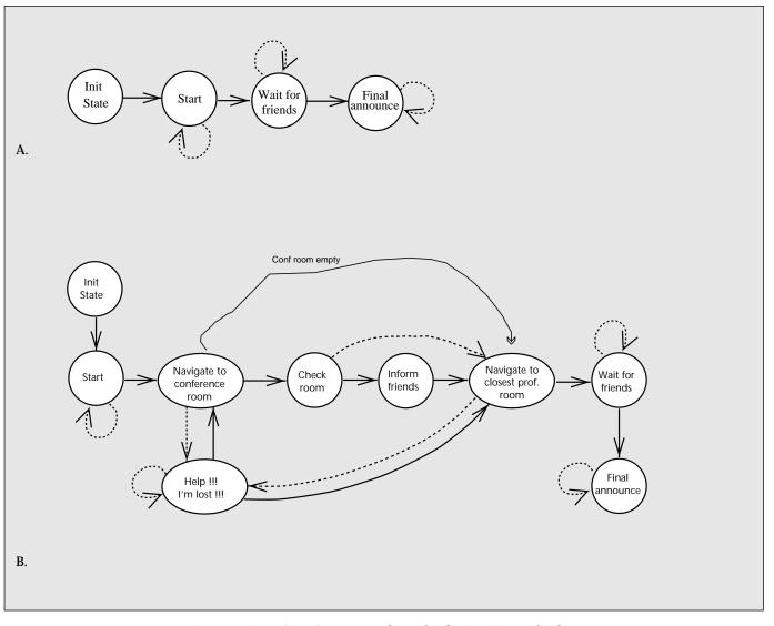
*Figure 7. Finite-State Strategy Machines for the Two Types of Robot.* A. Director's office robot. B. Traveling robot.
