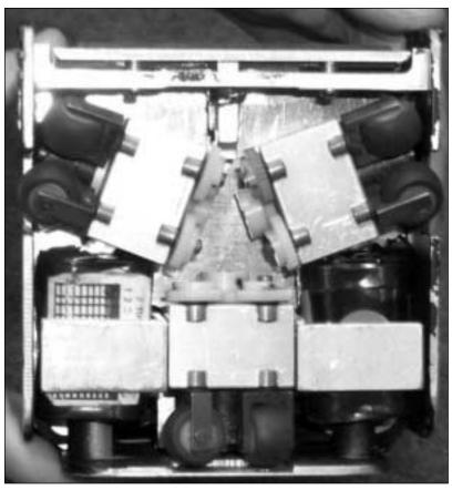
Figure 4. Bottom View, Omnidirectional Drive.
