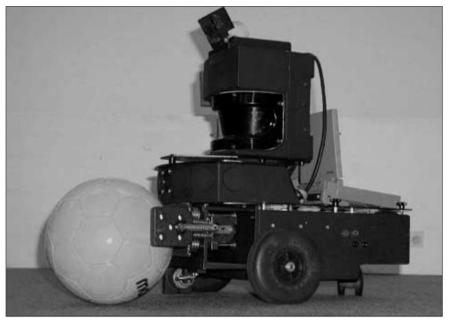
Figure 7. CS FREIBURG Player Mounting SICK LRF, Color Camera, Libretto Laptop, WAVELAN Wireless Ethernet, and Custom-Made New Kicking Device.
