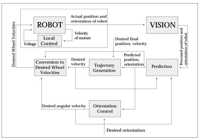
Figure 6. Block Diagram Representation of Trajectory Generation.
