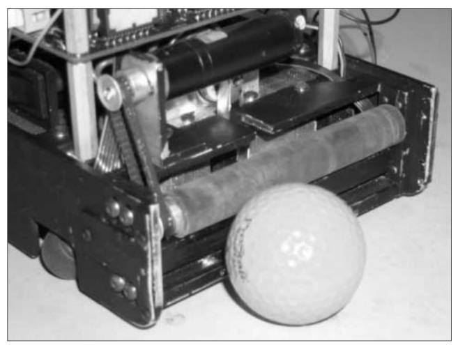
Figure 5. Angled View, Dribbling Mechanism.
