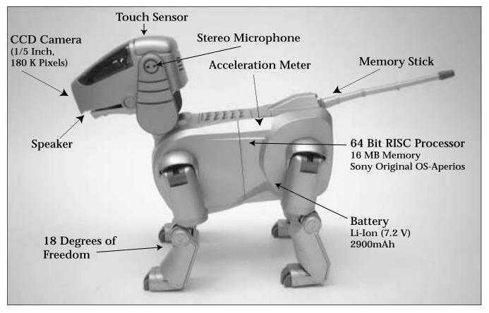
*Figure 1. The Legged Robot Platform.* Weight: 1.59 kg. Size: 2.75 x 156 x 266 mm (without tail).
