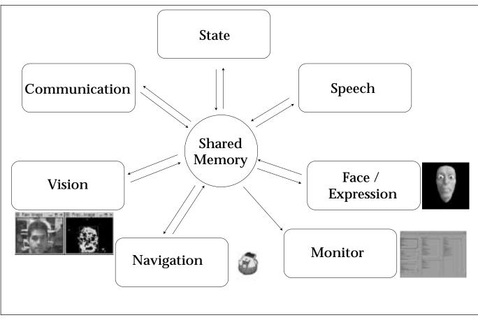
Figure 2. Logical Diagram of the REAPER Architecture.
