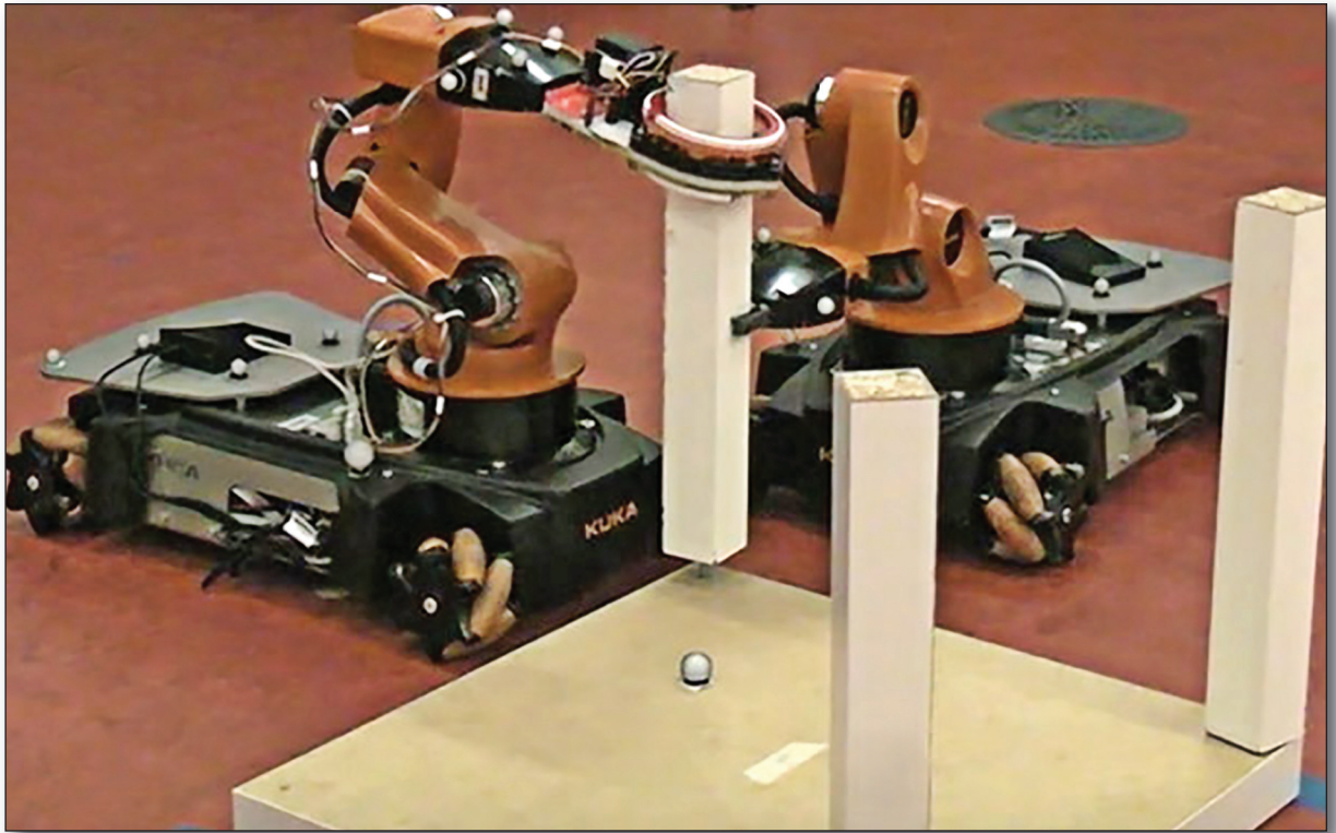
Figure 2. The IkeaBots Developed at the Massachusetts Institute of Technology Can Collaborate on the Construction of Modular Furniture.
