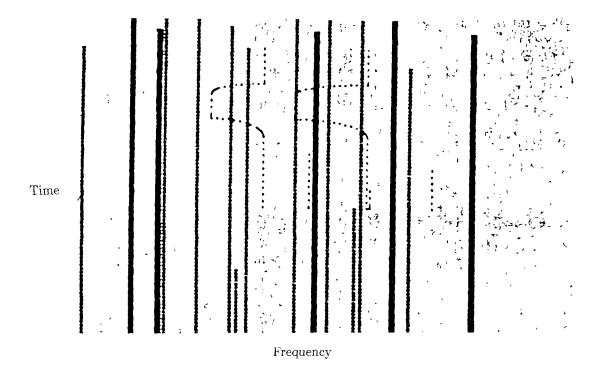
Figure 1. A simulated sonogram (with noise suppressed).
