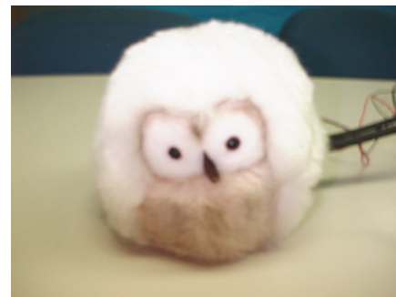
Figure 5: A stuffed puppet, which connects with a PC, has built-in sensors to detect tactile stimuli.
