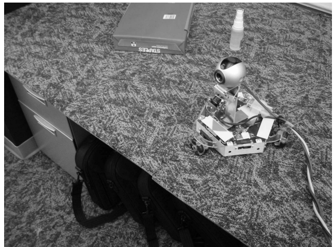
Figure 1: Robot poised near a drop-off to illustrate precipice detection. The visual navigation system demonstrated can reliably detect a cliff even when similar colors and textures appear at both the bottom and the top of the precipice (such as in this photo). The robot pictured has two cameras, but only the lower one, pointing roughly 30° below horizontal, is in use.
