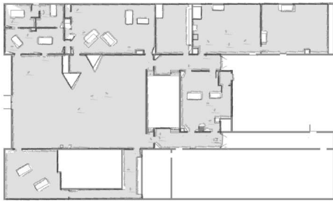
Figure 2: Generated map (free space in light gray) overlaid with a CAD model (in dark gray) of the building. The CAD model was generated from manual measurements by a third party. Map edges overlap in black.
