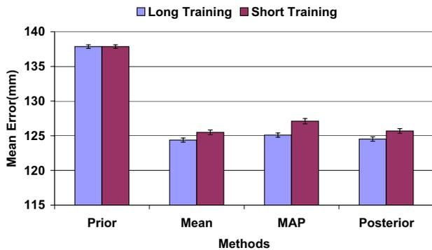
Figure 4: AIBO localization results with 95% confidence intervals.
