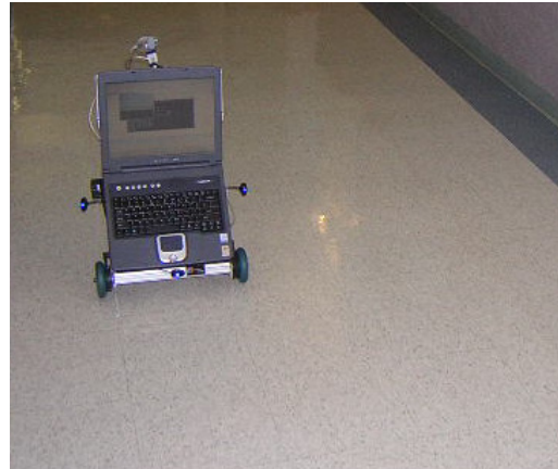
Figure 1: An Evolution ER1 robot with our current configuration. The USB camera and short range infrared sensors are both included with the ER1.
