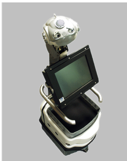
Figure 4: Pearl: A Mobile Robot Platform for the Autominder Cognitive Orthotic. Photo courtesy of Carnegie Mellon University.
