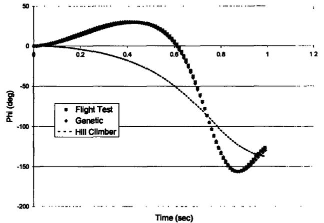
Figure 3. Euler Roll Angle Comparison
