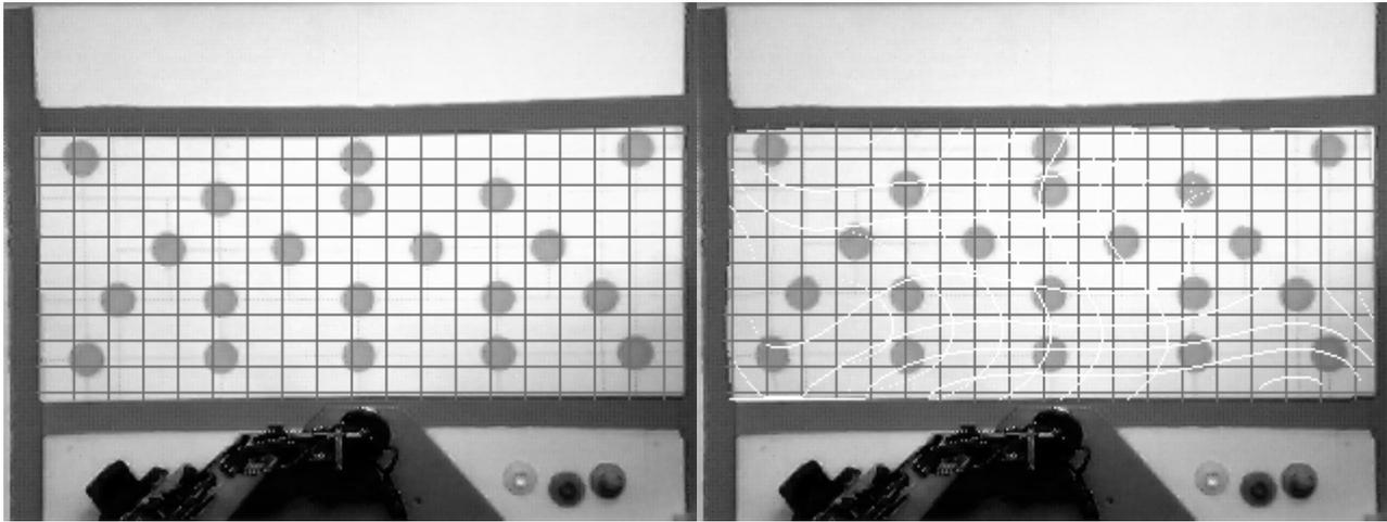
**Figure 2:** An unrectified image (left) and the corresponding rectified image (right). Only the region depicting the rectangular workspace was rectified and a grid was superimposed on this region to aid in comparison. The white streaks in the rectified image are “stretch marks”.
