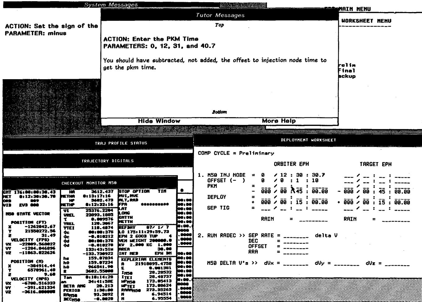
Figure 1. A typical screen as seen by a user of the PD/ICAT system. Menus at the upper right allow the trainee to interact with the system. Displays, identical to those used in the MCC, appear in the lower left. A worksheet used by the FDO in completing the task is shown in the lower right. System messages are displayed in the upper left, and error/help messages are provided in a pop-up window near the center of the screen.
