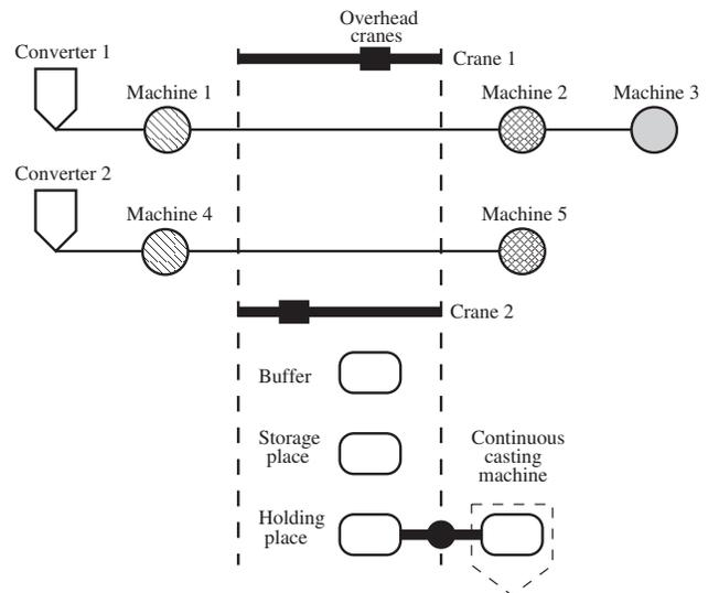
Figure 13: Layout of the SIDMAR steel plant.
