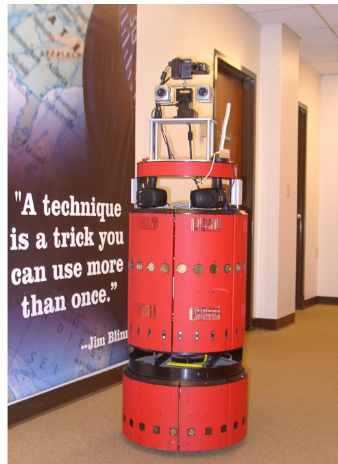
Figure 1: The experimental platform: Lewis, an iRobot B21r research robot
