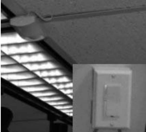
Figure 2: CASAS sensors: motion detector and Insteon light switch.
