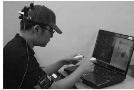
Fig 4. The Wearable Interface. The human operator is holding a Nintendo Wii Remote and a Nunchuk on both hands and wearing a set of 3DM-GX1 orientation sensors on both arms and the head.
