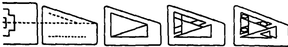
Figure 9. Design evolution: (1) axis extended from West Building, and setback lines, (2) diagonal divides 2 spaces, an isosceles triangle and a right triangle, (3) corners of isosceles triangle became exhibition towers, and (4) the right triangle became the Center for Advanced Study. (after (Galleries 1978))
