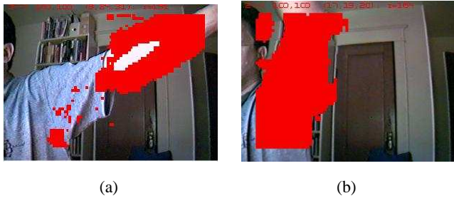
Figure 3: Dense Flow Estimate: (a) shows where optical flow vectors were detected using the Camus algorithm (Camus 1997), while (b) shows the result of motion detection based on only spatially propagating significant flow vectors.
