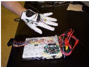
Figure 4: Second Generation Glove Prototype: of the tactile feedback unit is shown. There is a major compression of bandwidth in trying to convey a depth map in a tactile form on the hand. It is essential that an appropriate representation ease that transition.
