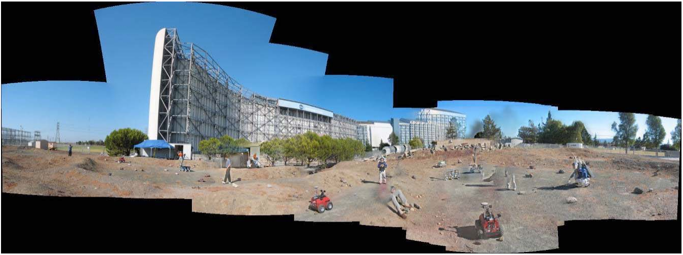
Figure 2: NASA ARC Human-robotic demonstration scenario, with single astronaut commanding two distinct rovers (K9, a highly autonomous MER class rover, and Gromit, a rapid robotic assistant) supported by habitat-based personnel.
