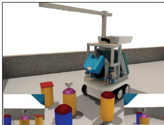
Fig. 5. Scenario of affordance based robot simulation experiments (Section III). Birds view illustrating robot Kurt2 within a scene of objects of colored cans, using a magnetic effector at the end of a rope for interaction with the scene, described in more detail in Section V. The lower left/right corner shows the field of view of the left and right camera, respectively.
