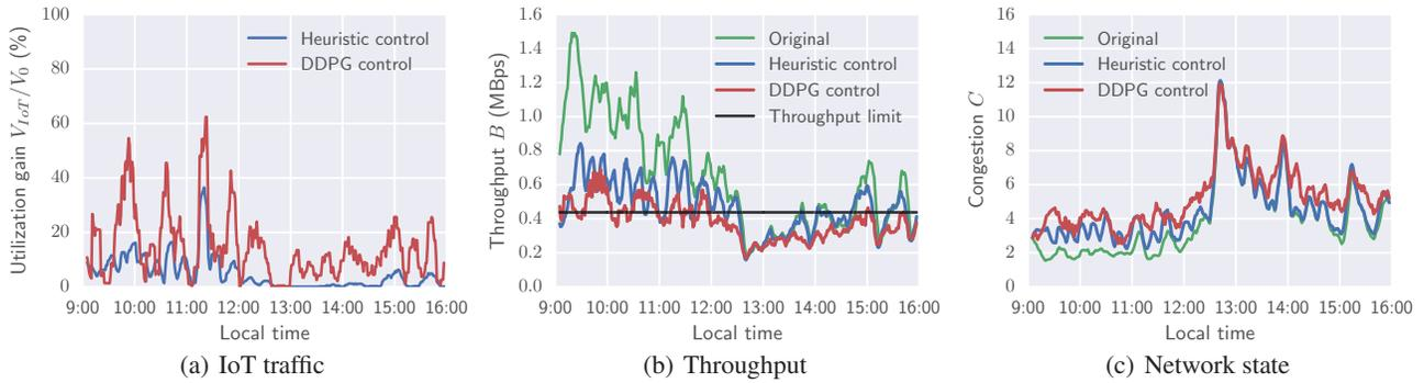
Figure 4: HVFT -RL smooths throughput variation and exploits transient dips in utilization in a Melbourne Cell.
