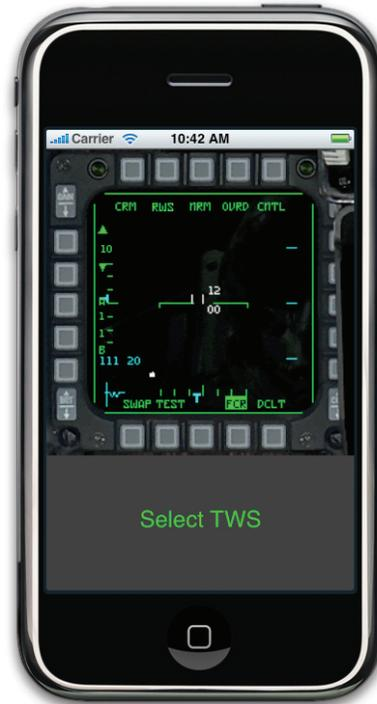
Figure 1: iPod prototype for Radar buttonology, with the hint *Select TWS* displayed
