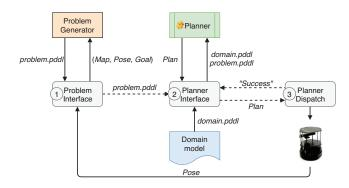
Figure 2: Pipeline of our energy-aware path planning package, where nodes are represented in gray and the service in yellow.
