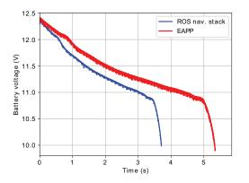
Figure 4: Battery discharge for the ROS navigation stack and the EAPP approach.
