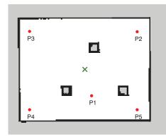
Figure 5: Map of the real world experiment environment, created with the SLAM package. The squares with black borders represent obstacles, red circles represent waypoints, and the green cross represents the center of the map, where the robot is initially positioned.
