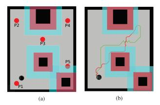
Figure 3: (a) Map used in simulation, where the red circles indicate the five waypoints. (b) Path planning considering the energy metric (green path) and ignoring the energy metric (red path). The simulated world consists of obstacles (black squares), the robot (black circle), and each obstacle's clearance and high energy zones (red and blue areas respectively). The walls also have these zones, omitted here for clarity.
