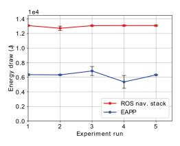
Figure 6: Energy draw with standard deviation for five experimental executions of the ROS navigation stack and the EAPP approach respectively, performing autonomous navigation for one hour in each execution.
