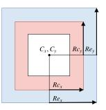
Figure 1: An obstacle, its clearance, and energy zones. The distances from the obstacle center to the boundaries of the red zone are the clearance radii, and the distances to the boundaries of the blue zone are the energy radii.
