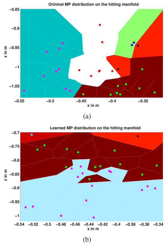
Figure 7: Distribution on the hitting manifold of the used motor primitives before (a) and after (b) training. Each color corresponds to one motor primitive in the movement library. Each point corresponds to the point of impact during evaluation.
