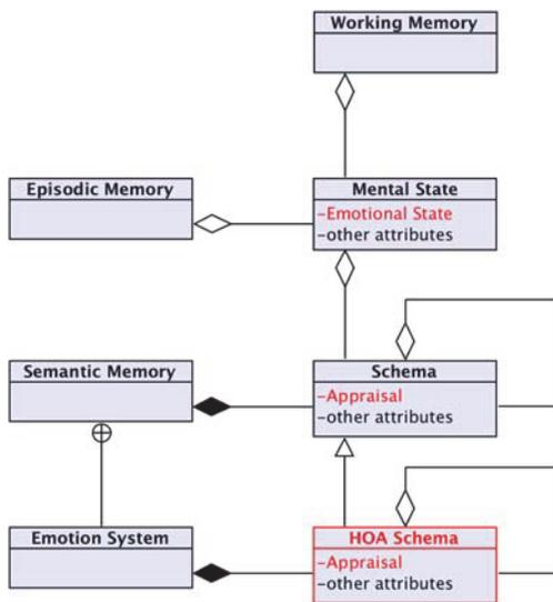
**Figure 5.** Essential core UML class diagram of the Constructor cognitive architecture extended to enable emotional intelligence. Emotional elements (shown in red) include two attributes (Emotional State, Appraisal) and higher-order appraisal (HOA) schemas. Appraisal values are shown in Figure 2. For details of the architecture, see (Samsonovich et al. 2006, Samsonovich 2009).
